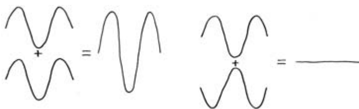
Constructive interference (bright)
